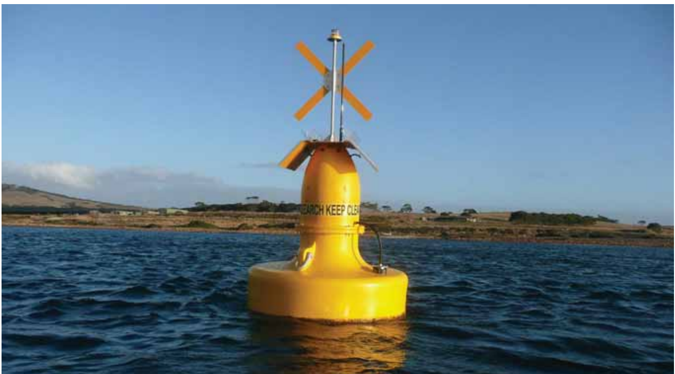
PLATE 9-2 WATER QUALITY MONITORING INSTRUMENT (YSI 6000) DEPLOYED IN SMITH BAY FOR ONE YEAR
